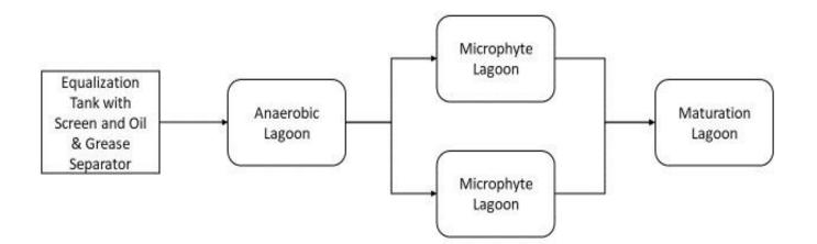
Anaerobic Lagoon: Usually deeper for anoxic conditions Facultative/Microphyte Lagoon: uses algae and ecosystem of bacteria, phytoplankton and bacteria Maturation Lagoon: to finish/polish effluent before discharge
